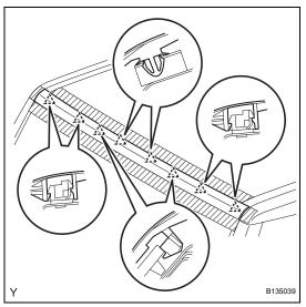
(d) Disengage the 6 claws and the 2 clips and remove the windshield outside upper moulding.
